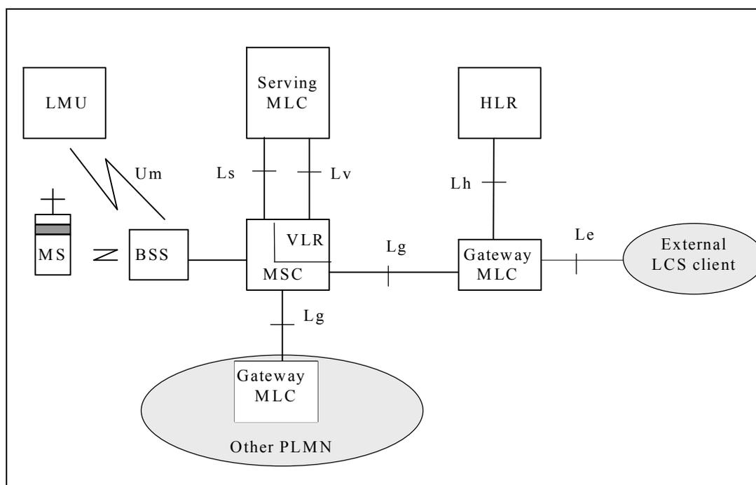
**Figure 4: Configuration of a PLMN supporting LCS**
