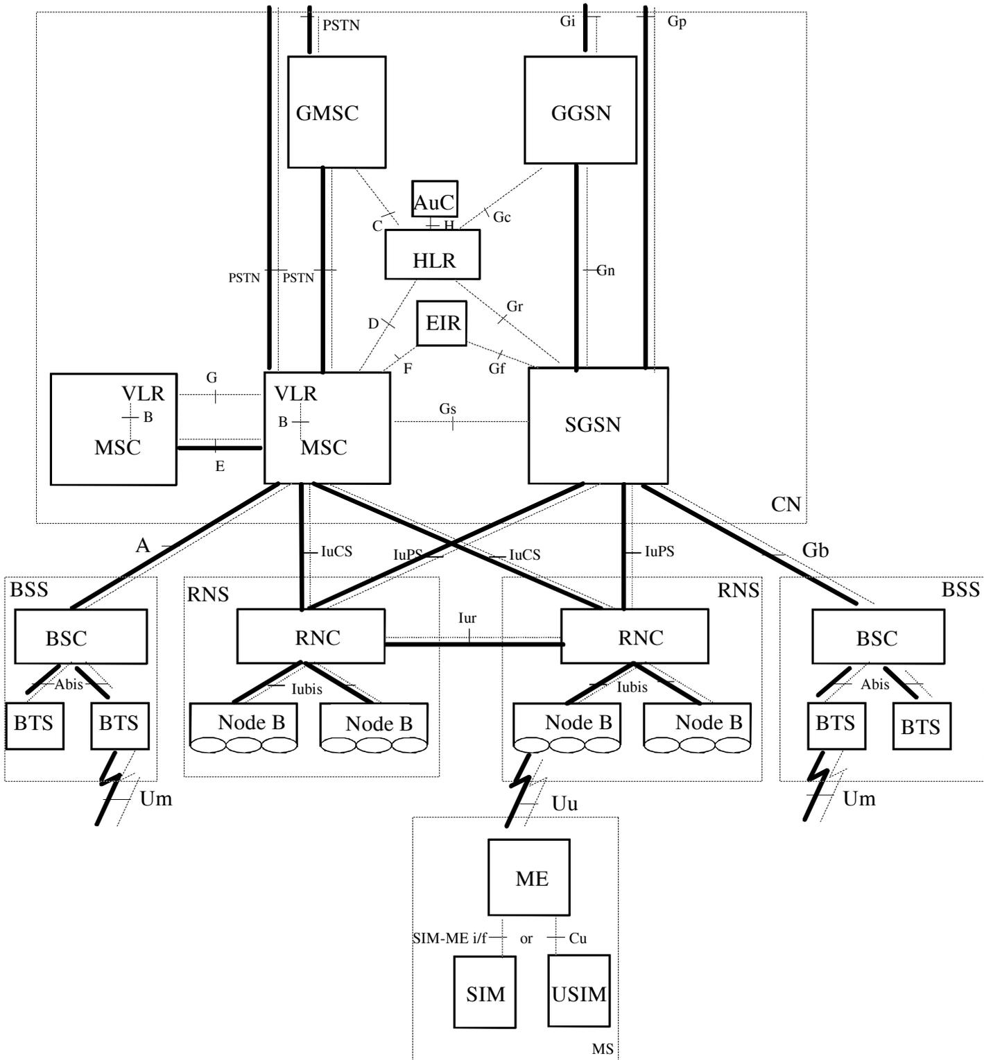
Figure 1: Configuration of a PLMN and interfaces
