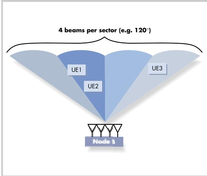
Space Division Multiple Access (SDMA) can be used to increase the downlink cell throughput by scheduling data packets simultaneously to users served by different beams. This limits mutual interference between these users, making it possible to reuse the same channelization code resources. SDMA implementation requires extensions to the MAC-hs packet scheduler to enable the spatial separation of users and possibly code reuse. *Figure 3* shows a possible transmission scenario
